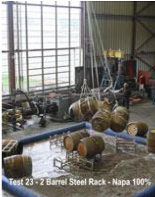
Barrels stacked on steel racks would only pass 75% Napa quake energy. Photos: UC Berkley PEER Test Center
