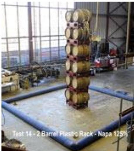
Barrels stacked 6 high on plastic racks after 125% of Napa quake energy.
